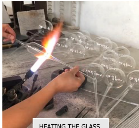
HEATING THE GLASS
