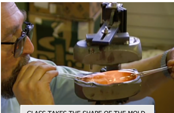
GLASS TAKES THE SHAPE OF THE MOLD
